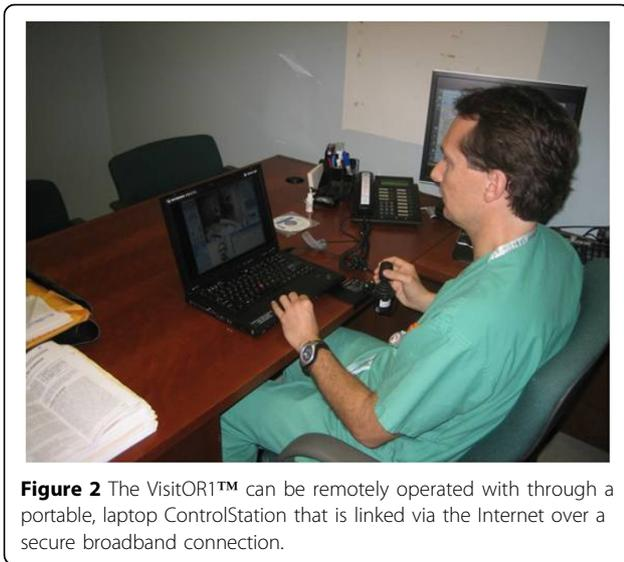
**Figure 2** The VisitOR1™ can be remotely operated with through a portable, laptop ControlStation that is linked via the Internet over a secure broadband connection.
